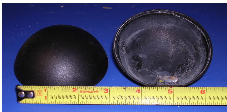
Figure 4.13. Mold used by Puryear (2007) to fabricate fiber-reinforced cement paste housing (3.5-in. diameter and 1.5-in. high).
