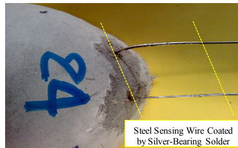
Figure 4.33. Photograph showing the solder coating on the surface of sensing wire.
