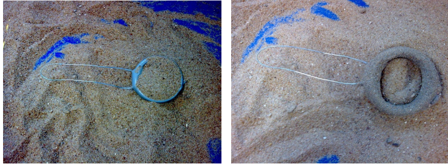
Figure C.4. The process to increase the roughness of the epoxy housing surface.
