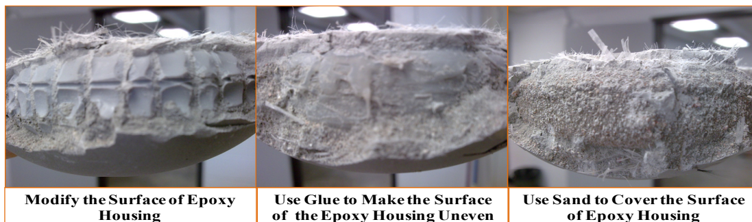
Figure 4.31. Three methods used to increase the roughness of the epoxy coating.
