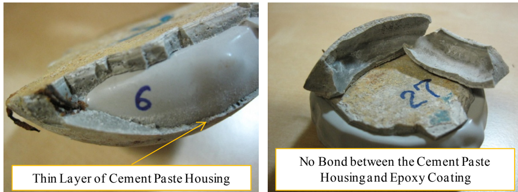
Figure 4.21. Photographs of the interface between the cement paste housing and the epoxy coating (Sensors J006 (left) and J027 (right)).
