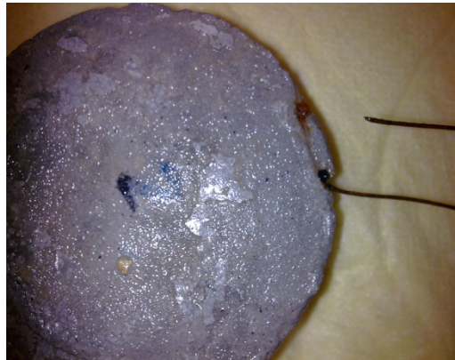
Figure 4.17. Steel sensing wire fractured at the outer face of the cement paste housing for Sensor J002.
