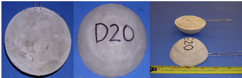
Figure 4.6. Photographs of sensor with fiber-reinforced cement paste housing (Puryear 2007).
