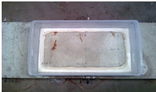
Figure 3.7. Photograph of the salt-water reservoir positioned at the midspan of Slab 3 (Puryear 2007).
