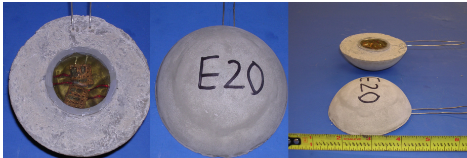
Figure 4.7. Photographs of sensor with fiber-reinforced cement paste housing and epoxy core (Puryear 2007).
