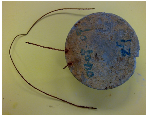
Figure 4.18. Steel sensing wire fractured along the free length (Sensor J027).
