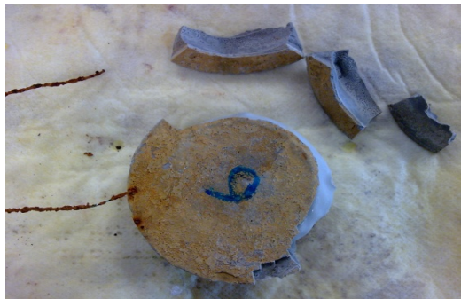
Figure 4.30. Photograph of cement paste housing at the conclusion of the first accelerated corrosion test (Sensor J006).
