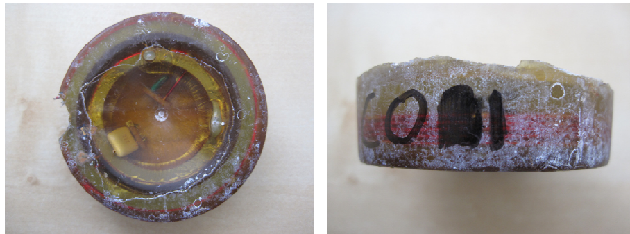
Figure 3.26. Top (left) and side views (right) of corrosion products in Sensor C01.
