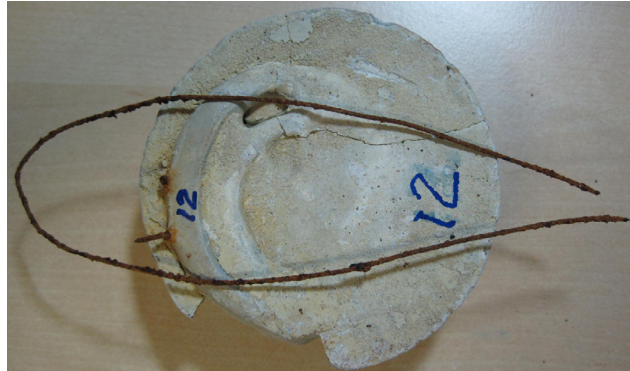
Figure 4.23. Uniform corrosion of the steel sensing wire for sensors that were not completely encased in the cement paste housing (Sensor J012).
