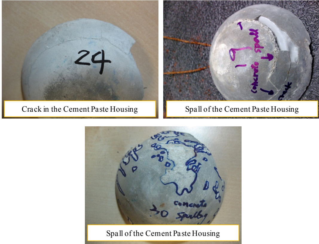
Figure 4.20. Photographs of cement paste housing at conclusion of accelerated corrosion test (Sensors J024 (top-left), J019 (top-right) and J003 (bottom)).
