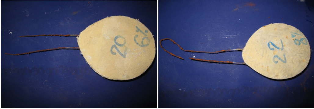
Figure 4.43. Condition of cement paste housing at conclusion of second accelerated corrosion test for Sensor N020 (left, 6% salt water) and N022 (right, 8% salt water)
