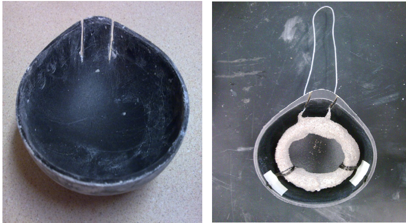
Figure 4.29. Two grooves in the new mold (left) allow the potting to proceed without bending the steel sensing wire (right).
